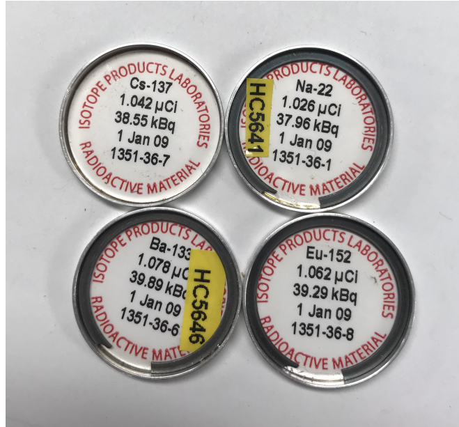
Figure 4.8: The calibration sources that were used in this efficiency calibration of the detector (Na-22 was not used in the calibration). Picture from private communication with Hannah Ekeberg.
