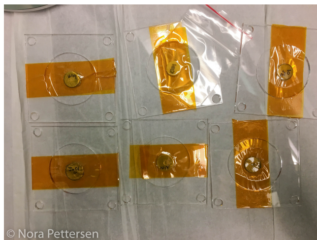
Figure 4.11: Picture of how the targets were sealed before irradiation. From the top left to right: Zn, NaCl, Zr and bottom left to right: In, Y, Al. The NaCl target was there for a different experiment.
