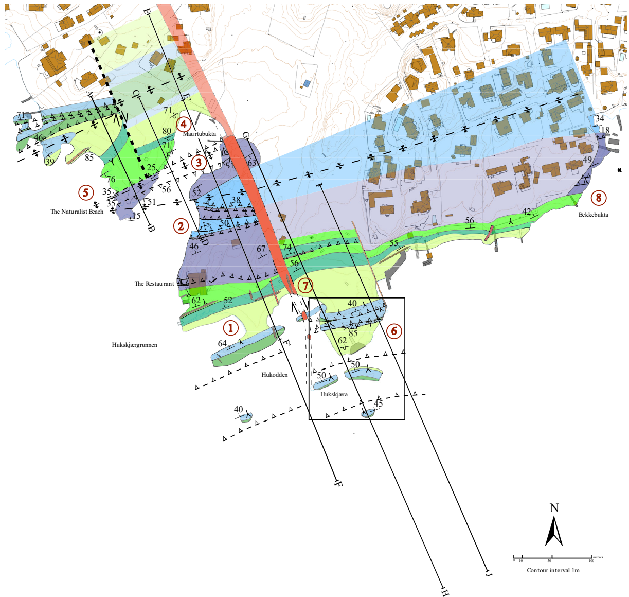
Figure 5.2.1: Geological map of the Huk area of southern Bygdøy. A major, vertical, NNW-SSE trending syenite porphyry dyke of Permian age cuts through the area. Sub-areas are marked by encircled numbers. Black box marks detailed map of Sub-area 6 (Fig. 5.2.7.1). Colours and symbols explained in legend found in Figure 5.2.2. The map is also found in Appendix 3 (Plate 1), where more measurements are included.
