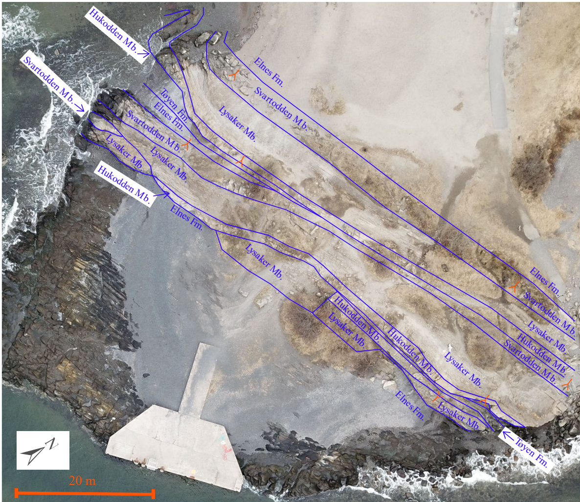
Figure 5.2.7.2: Drone photo of the Hukodden imbricate structure. The boundaries between lithological units, as well as the name of the units have been marked in dark blue. Right way up indicators are included in orange, but faults, other structures, and measurements have not been marked on the figure. Figure can also be found in Appendix 3 (Plate 12).
