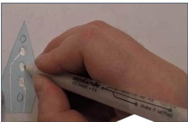
I drew circuits and connection points with conductive ink on post-it notes. The result felt elegant and light.
