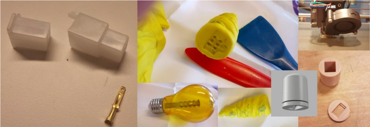
Figure 16 Prototype of Socket Connector; f.l. male/female connector, play-dough socket connector, light bulb inspiration, 3D-rpinting a casing
