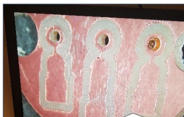
I inspected the PCBs through a microscope to make sure the paths were clear of copper
