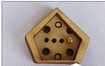
and cut small holes in the Finnwood with the laser cutter, just wide enough to hold the tiny pogo pins
