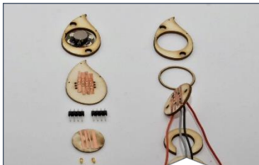
I experimented with creating the casing and the circuit boards with Finnwood, a very light and sturdy form of cardboard, both for the casing and as the electronic interior.
