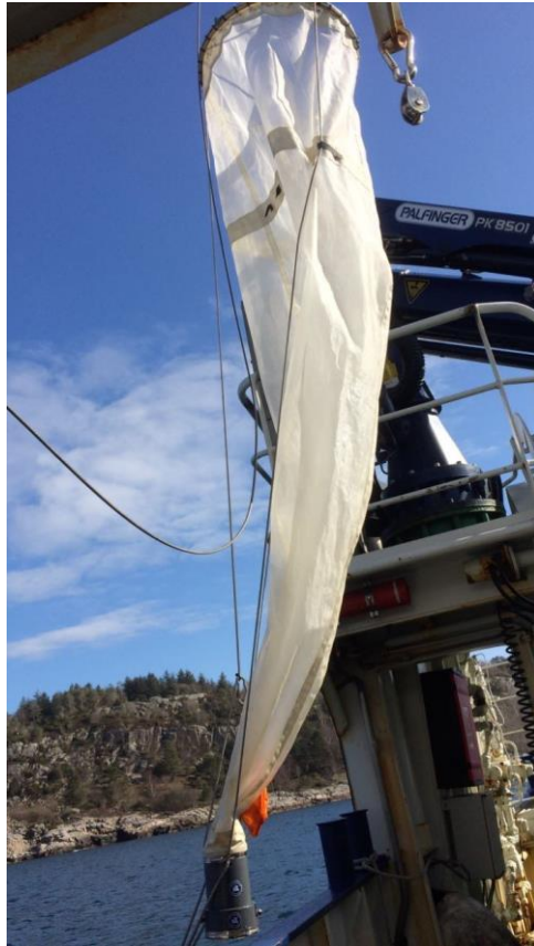
Figure 7. Picture of the egg net used during the cruise. On the bottom of the net is the detachable cup and the Cast-Away CTD.
