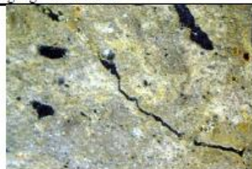
Fig. 5: As Fig 4, under OIL; note general lack of iron staining.
