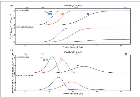
**Figure A3.** Graphical representation of equations (A.14) and (A.18) for various  $t_{\rm illum}$ . Results are shown for (a) conventional and (b) derivative SSPC spectra. Here, the  $\sigma_{\rm n,norm}^{\rm o}$  calculated for  ${\rm Ti}_{\rm GaII}^{+/0}$  was used. Moreover, the following parameters were used:  $\Delta E=20~{\rm meV}, \Sigma_{\rm n}^{\rm o}=2\times 10^{-20}~{\rm m}^2, \Phi=1\times 10^{18}~{\rm m}^{-2}~{\rm s}$  and  $N_{\rm tr,eff}^{\rm ss}=1\times 10^{16}~{\rm cm}^{-3}$ .
