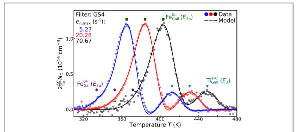
Figure 3. DLTS spectra recorded on a EFG-grown  $\beta$ -Ga<sub>2</sub>O<sub>3</sub> crystal. The DLTS spectra were constructed with a GS4 filter and compared to simulations (solid lines). Three defect signatures  $Fe_{Gal}^{0/-}(E_{2a})$ ,  $Fe_{Gall}^{0/-}(E_{2b})$  and  $Ti_{Gall}^{+/0}(E_3)$  are observed and labeled.
