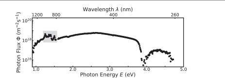
**Figure 1.** Photon flux  $\Phi(E)$  recorded for the optical excitation used for SSPC measurements. A structure is marked in gray which also appears in SSPC measurements.
