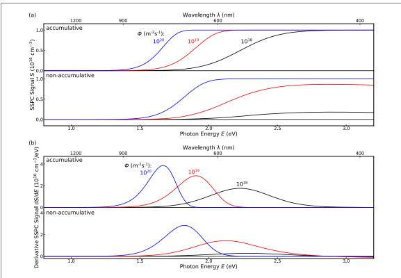
**Figure A2.** Graphical representation of equations (A.14) and (A.18) for different photon fluxes  $\Phi$ . Results are shown for (a) conventional and (b) derivative SSPC spectra. Here, the  $\sigma_{n,norm}^{o}$  calculated for  $\mathrm{Ti}_{GaII}^{+/0}$  was used. Moreover, the following parameters were used:  $\Delta E = 20$  meV,  $\Sigma_{n}^{o} = 2 \times 10^{-20}$  m<sup>2</sup>,  $t_{illum} = 10$  s and  $N_{tr,eff}^{ss} = 1 \times 10^{16}$  cm<sup>-3</sup>.
