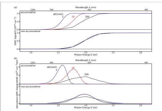
**Figure A4.** Graphical representation of equations (A.14) and (A.18) for various  $\Delta E$ . Results are shown for (a) conventional and (b) derivative SSPC spectra. Here, the  $\sigma_{n,norm}^o$  calculated for  $Ti_{GaII}^{+/0}$  was used. Moreover, the following parameters were used:  $t_{illum} = 300 \text{ s}$ ,  $\Sigma_n^o = 2 \times 10^{-20} \text{ m}^2$ ,  $\Phi = 1 \times 10^{18} \text{ m}^{-2} \text{ s}$  and  $N_{tr,eff}^{ss} = 1 \times 10^{16} \text{ cm}^{-3}$ .
