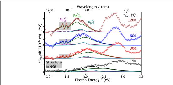
$\textbf{Figure 5.} \ \ \text{Accumulative SSPC spectra recorded on a EFG-grown } \beta \text{-} Ga_2O_3 \ \text{crystal using different } t_{illum}. \ \text{The spectra were modeled}$ with equation (6), and the models are shown in solid lines. The model parameters are shown in table 2. A feature related to the spectral shape of  $\Phi$  is marked in gray (see figure 1).
