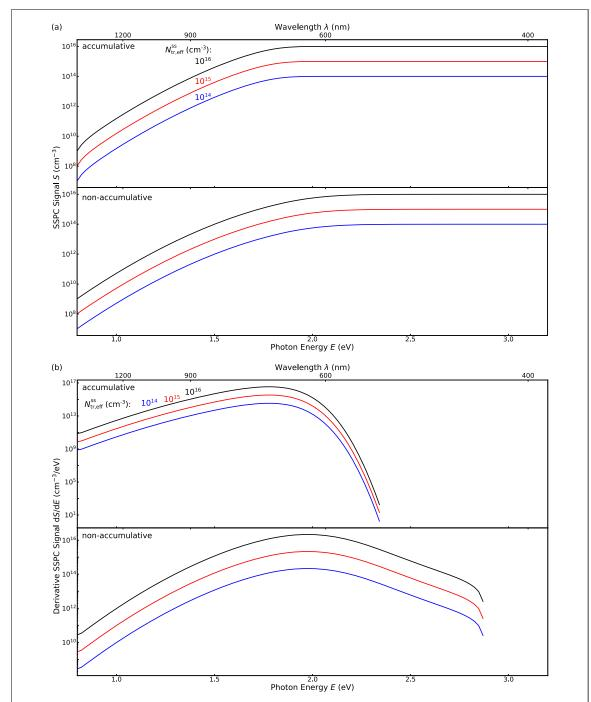
**Figure A5.** Graphical representation of equations (A.14) and (A.18) for various  $N_{\rm tr,eff}^{\rm ss}$ . Results are shown for (a) conventional and (b) derivative SSPC spectra. Here, the  $\sigma_{\rm n,norm}^{\rm o}$  calculated for  ${\rm Ti}_{\rm GaII}^{+/0}$  was used. Moreover, the following parameters were used:  $t_{\rm illum}=300~{\rm s}, \Sigma_{\rm n}^{\rm o}=2\times 10^{-20}~{\rm m}^2, \Phi=1\times 10^{18}~{\rm m}^{-2}~{\rm s}$  and  $\Delta E=20~{\rm meV}$ .
