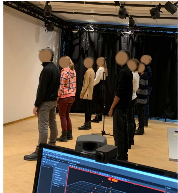
Figure 1: A group of participants ready to stand still. Each participant wears a motion capture marker on top of their head. A reference marker placed on a tripod can be seen between the participants. Two speakers in front of the participants were used for sound playback.
