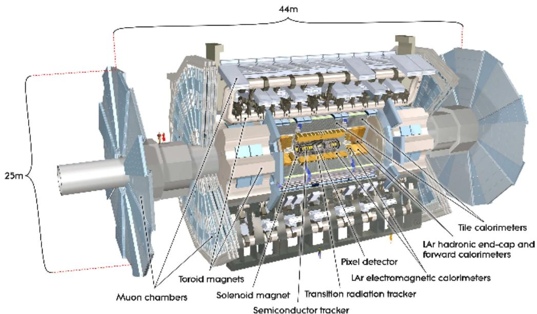
Figure 2.2: An illustration of the ATLAS detector [18].
