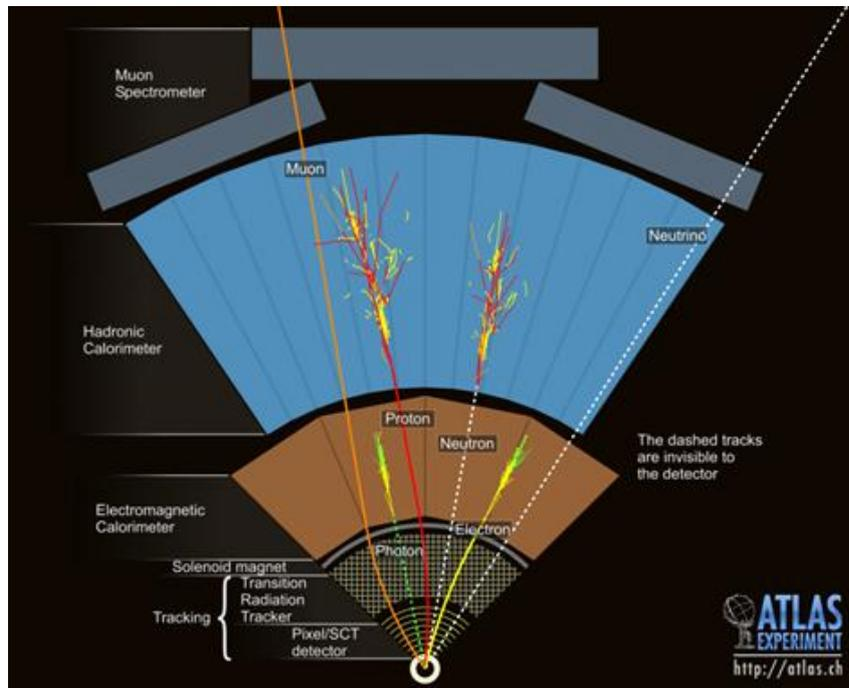
Figure 2.3: An illustration on how we see the tracks of the different particles in the detector [19].
