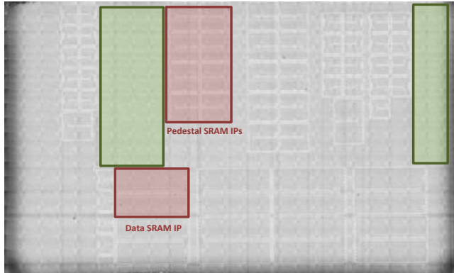
Figure 3-2 inspected zones on SAMPA "V4"
