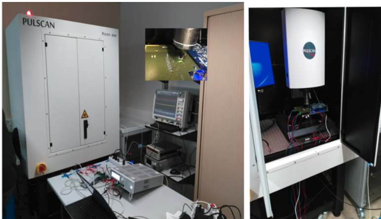
Figure 6.16: SAMPA test setup connected to the PULSYS-RAD system during the pulsed-laser campaign.
