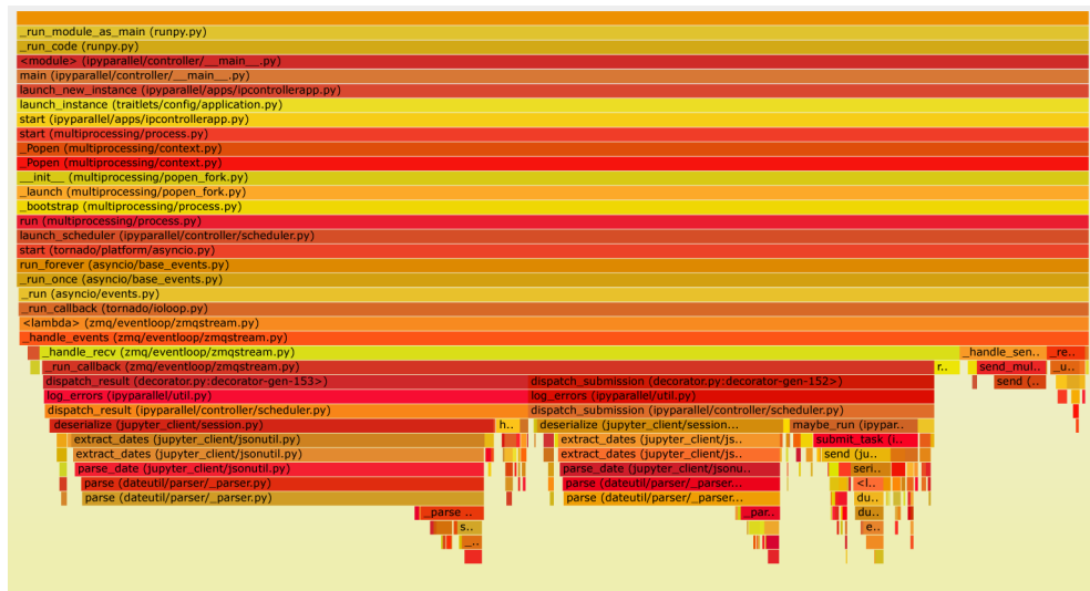
Figure 4.4: Profiling execution of LoadBalanced.apply on the task scheduler
