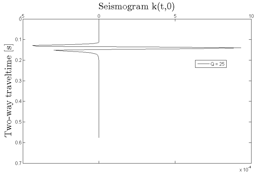
FIGURE 3.11: Forward modelled seismogram, k(t,0) using Q = 25 .
