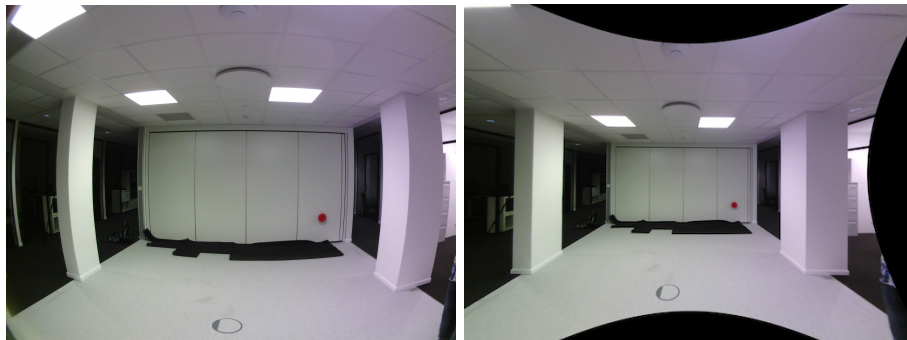
Figure 4.4: Before (left) and after (right) distortion correction is applied to the raw image from the camera.
