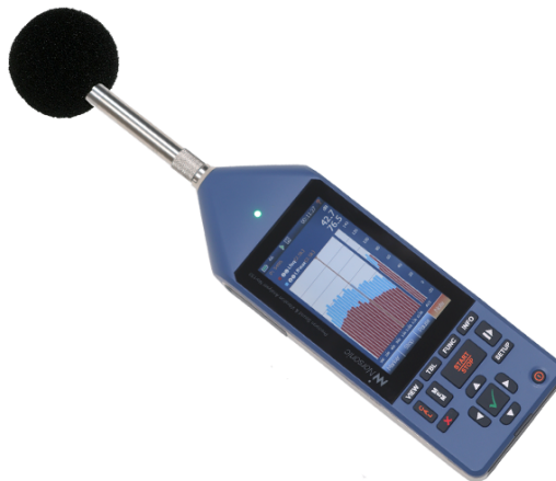
Figure 1.1: Sound level metre used to measure noise pollution, building acoustics and environmental noise. Image taken with permission from norsonic.com
