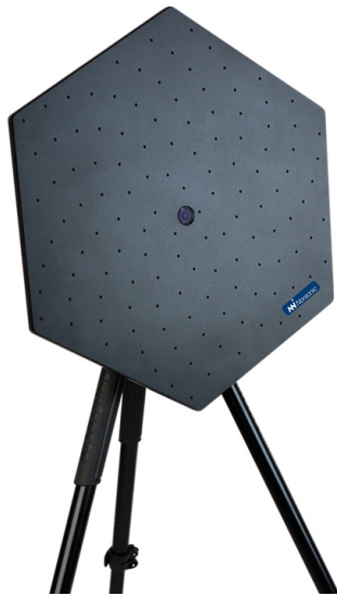
Figure 2.1: The Hextile Acoustic Camera microphone array used in experiments
