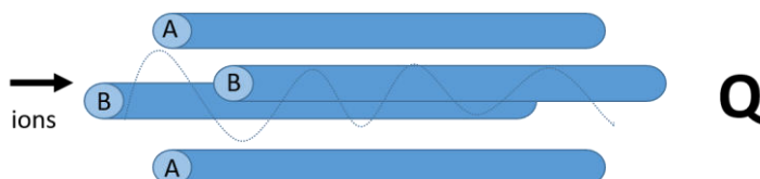
Figure 14. Schematic representation of the Q analyzer: two pairs of metal rods (A and B) in square configuration.
