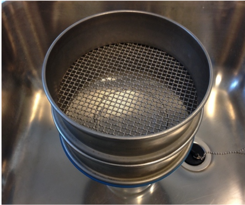
Figure 5. 5mm metal filter stacked on 1mm filter with a glass beaker beneath
