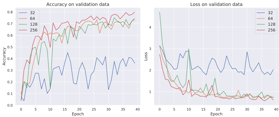
Figure 4.11: Model accuracy and loss measured on the validation dataset during training. Blue: 32 \times 32 , Orange: 64 \times 64 , Green: 128 \times 128 and Red: 256 \times 256 .
