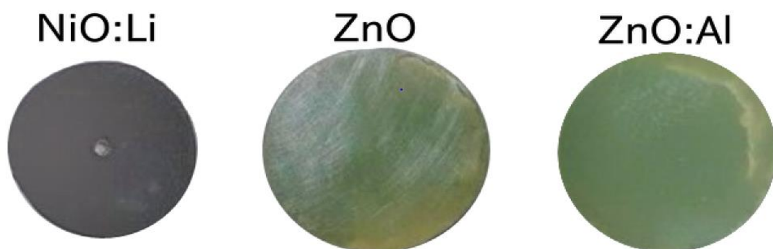
Figure 27: Pellets produced from powders, from the left is NiO:Li, ZnO, and ZnO:Al.
