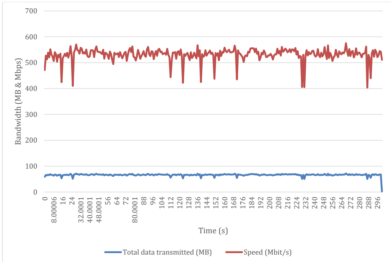
Figure 69. Software-Defined VPN single-stream tests over the SR-IOV virtualization plane between 5GC and CU.
