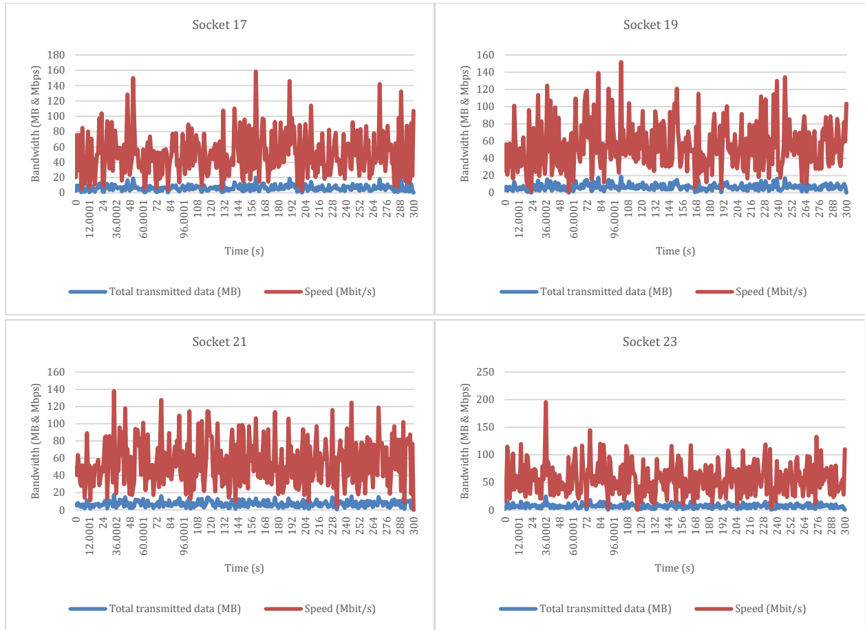
Figure 68. Last four socket streams from the multi-stream VPN hardware-level tests.
