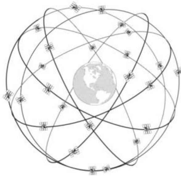
Figure 2.9: A network of GPS satellites consisting of 24 operational satellites in six orbit planes (reprinted from Dzurisin, 2007).
