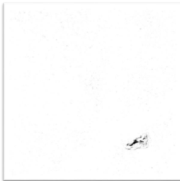
Figure 3.6: Greyscale correlation map of the digital image correlation of the selected area of study. Darker shades correspond to poor correlation, and lighter shades correspond to good image correlation. Optimally these maps should be as white as possible. Notice the dark patch at the right edge of the figure. This is where the oil has erupted. The oil is transparent and reflective, which creates difficulties for the image correlation resulting in a bad correlation value.
