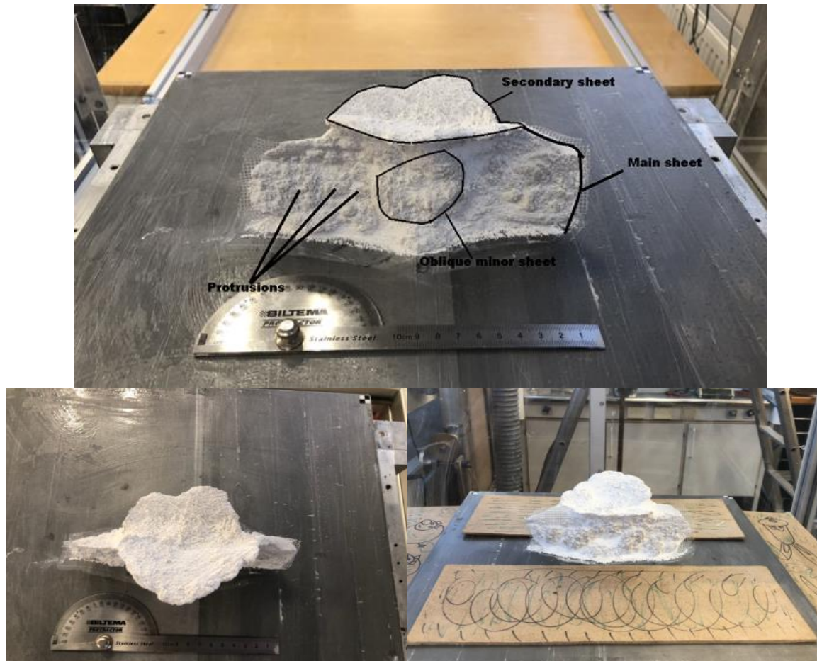
Figure 4.1: Examples of the final geometry of an excavated intrusion using an 8 cm net. Intrusion characteristics are outlined and marked in the upper image. The lower left is a top view, and the lower right is the back view.
