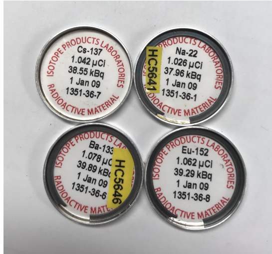
Figure 3.5: The calibration point sources that were used in the efficiency calibration of the detector. ( ^{22}\text{Na} was not used as part of the efficiency calibration due to its presence in the counting room background).
