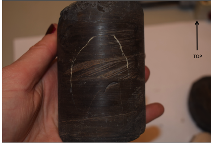
Figure 5.4: Steeply dipping calcite veins, with an aperture of 1 mm to 2 mm, from the Rurikfjellet Formation. The vein was situated at 383 m depth in DH4. The diameter of the core is 78 mm.
