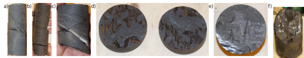
Figure 3: Photos from the fracture analysis. a) DH2 658.84m, b) DH2 659.95m, c) DH2 678.85m, d) DH2 675.84m, e) DH4 382.99m and f) DH4 439.64m. a) displaying a fracture of higher angle cutting two sub horizontal fractures. b) and c) displaying calcite veins and d-f) displaying slip surfaces, which are partially polished slickensides. Core is 5cm in diameter.
