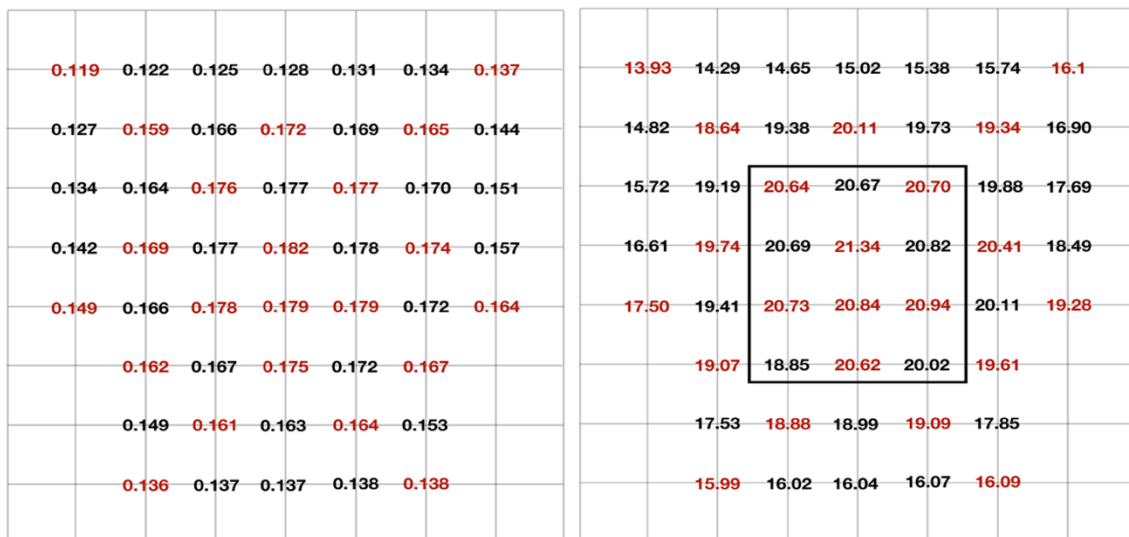
Figure 4.1: Ionization chamber measurements. Values in red were measured using the chamber, values in black were found from a linear interpolation. Left image shows the current detected, and right image shows the charge measured after one minute of irradiation.
