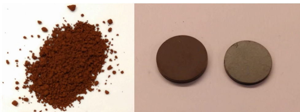
Figure 5-4: \text{Ca}_3\text{CoMnO}_6 powder to the left and two pellets of \text{Ca}_3\text{CoMnO}_6 sintered at a) 1050 °C and b) 1200 °C. The colour change from red/brown to grey was observed when \text{Ca}_3\text{CoMnO}_6 was treated at a higher temperature than 1100 °C.
