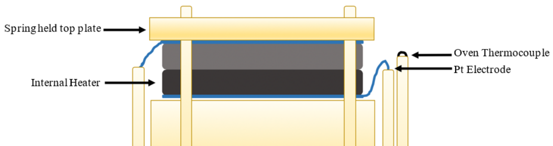
Figure 4-5: Illustration of the experimental setup for the measurement of stacks of CMO and CCO with a CCMO thin-film. The top of each outer surface is painted in Pt paint before adding a Pt mesh connected to the electrodes. The stack is held in place with a spring-loaded alumina top plat. The temperature of the oven is controlled by the external thermocouple
