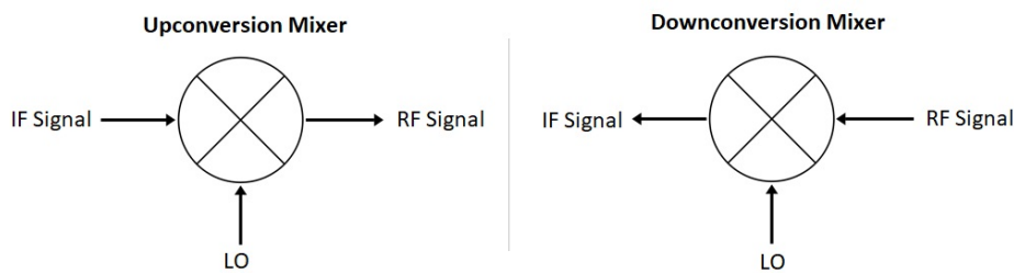
Figure 2.4: Mixer used for the transmitter unit (left) and for the receiving unit (right)
