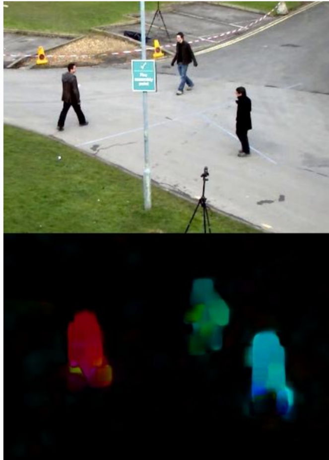
Figure 3.6: The top image shows the scene that is computed. The bottom image of the figure shows the results of computing dense optical flow between two images [64].
