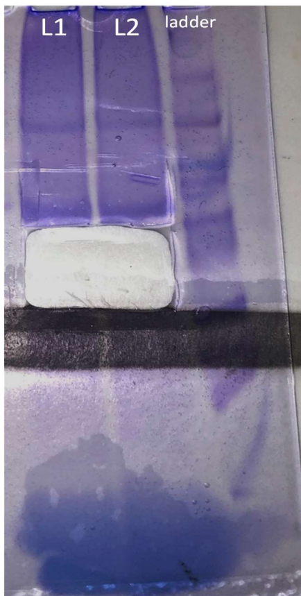
Figure 55: Gel electrophoresis - gel slab of two lanes of 60 \mu L lysed hepatic organoids in each well (L1, L2) compared to protein ladder reference. The reference could not be used as an overload of the wells for the hepatic organoids morphed the lane for the protein ladder. The excision of slabs for ALT1 were based on the bold band for the sample lanes, which was assumed to be from HSA (66.5 kDa), being the most abundant protein in organoids. The excised bands from both lanes were pooled to increase analyte abundance in the analyzed sample.
