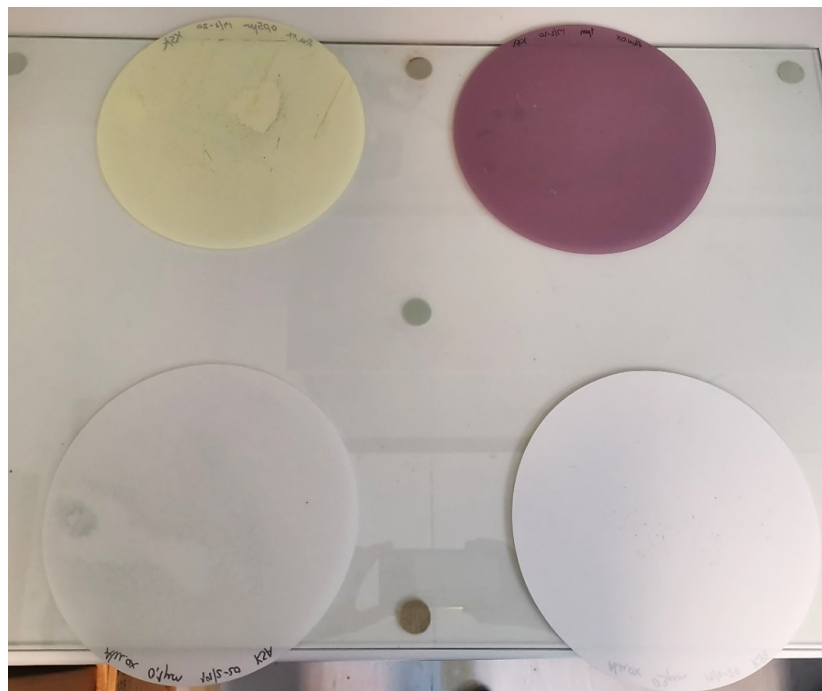
Figure 4.7: Polishing papers from Struers glued to a glass plate as described in the third polishing method. Starting in the upper right corner, going clockwise, from coarsest to finest grains.
