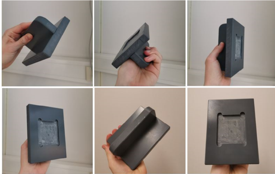
Figure 4.6: The sample holder for polishing, which was custom-made for this study. It is made to hold the 5 x 5 cm 2 glass samples in place when polishing their surfaces.
