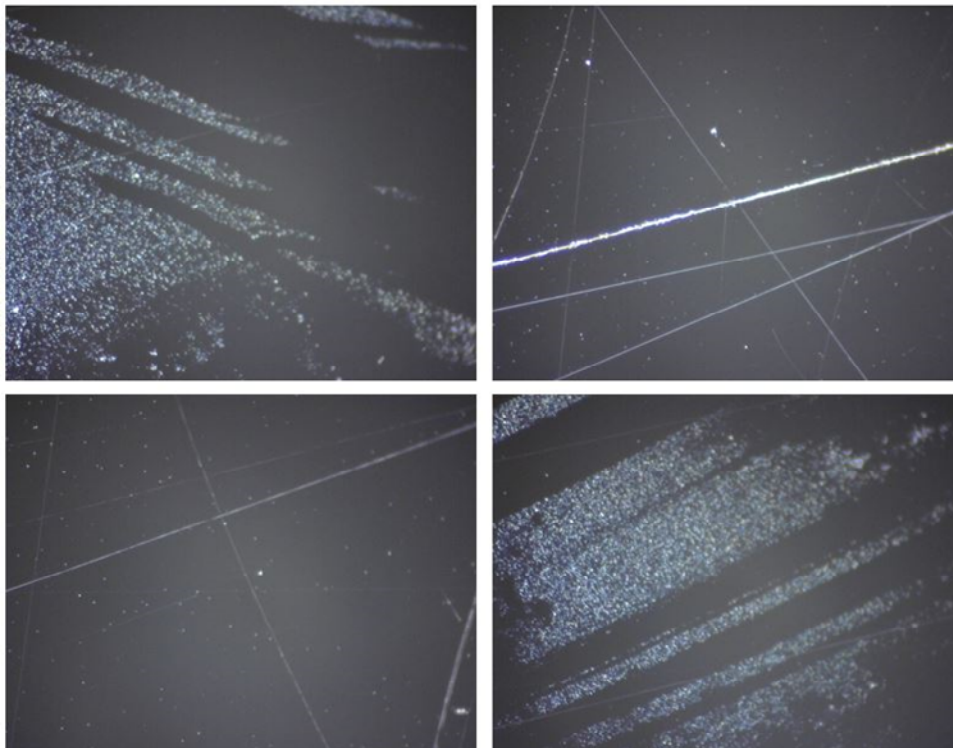
Figure 8.4: USB-microscopy photos of sample F1L, polished by hand with 0.1 μm diamond suspension with visible suspension remains at x778 magnification.
