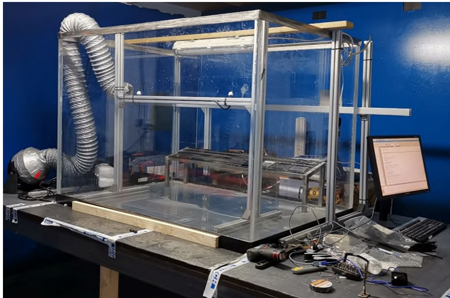
Figure 8.8: Custom-made test box, made for exposure experiments of seawater. Was not used due to external circumstances.
