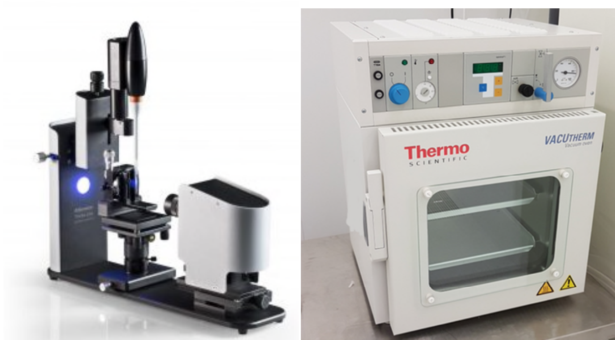
Figure 4.4: Left: Biolin Scientific Attention Theta Lite optical tensiometer used for measuring contact angles in this work. Right: VACUtherm furnace from Thermo Scientific used for the coating process by evaporation. The images are reproduced from the distributors.
