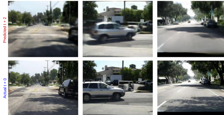
Figure 2.14: PredNet predicting two frames into the future of a dashboard camera video sequence. Adapted from Lotter et al. (2016).
