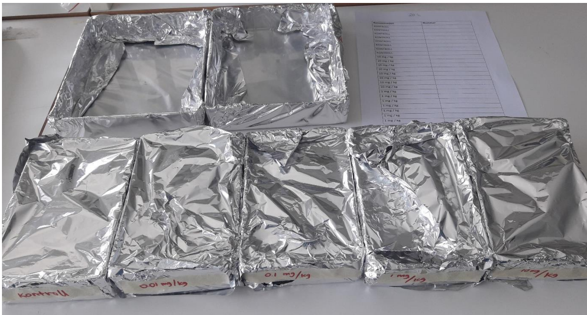
Picture 6: Blinding and randomization of the boxes with soil. The larger containers are packed in aluminium foil to prevent any degradation of imidacloprid by light.
