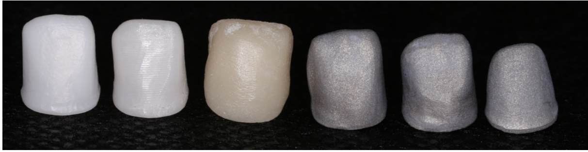
Figure 6. Test specimens used in this thesis. From left to right; zirconium dioxide, HIP zirconium dioxide, lithium disilicate reinforced glass ceramic, milled cobalt-chromium, sintered cobalt-chromium, and cast cobalt-chromium
