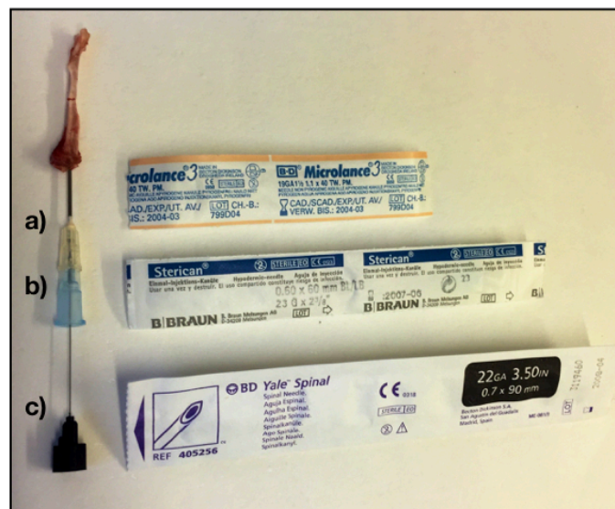
Figure 10. Components of the nail as tested in the cadaveric pilot study. a) Outer cannula: 23G 0.6x60 mm Sterican, Braun, Germany. b) Middle cannula: 19G 1.1x40 mm Microlance3, BD, Spain. c) Inner mandrin: Spinal needle, the stylet only. 22G 0.7x90 mm Yale Spinal, BD, Spain.
