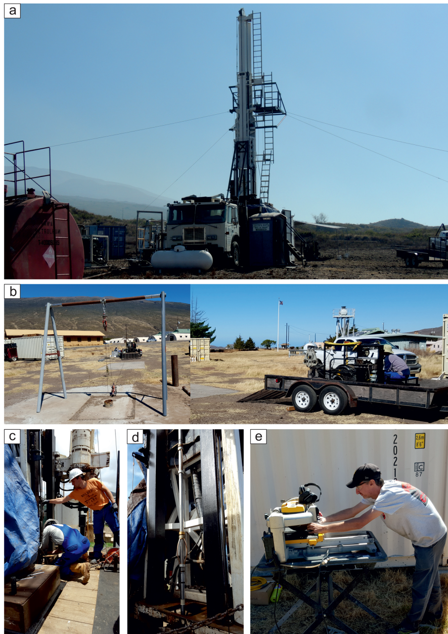
Figure 2. (a) Drill truck at the KMA1 site. (b) Spectral gamma logging within casing at PTA2. (c) Jochem Kück and Marco Groh (GFZ) with the sonic sonde at PTA2. (d) Borehole televiewer sonde being lowered into the borehole at PTA2. (e) Eric Haskins cuts sections of core for additional sampling.
