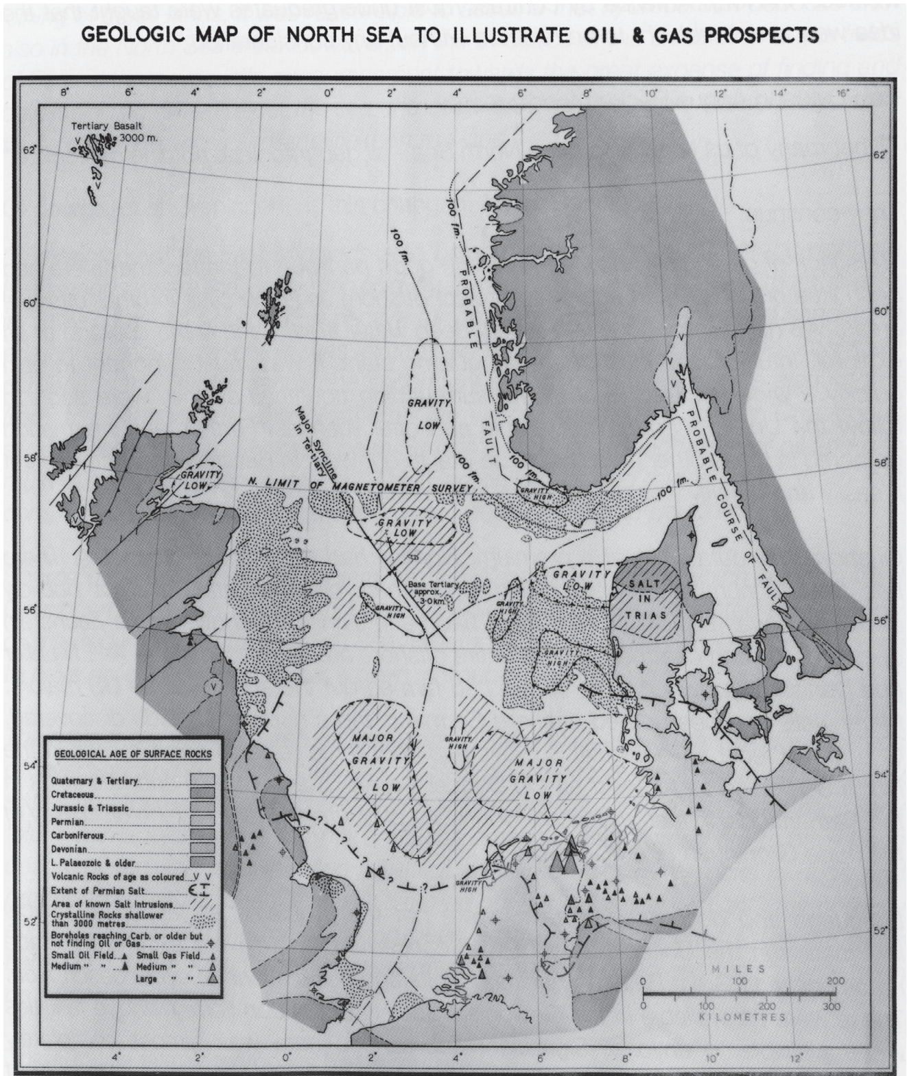
Figure 1. Early geological map of the North Sea, 1962–1963. Salt had been detected from gravity and magnetic surveys, but there was little information about North Sea rifting. This provided only a limited basis for prediction of the petroleum potential. From Moreton (1995). Reproduced with permission from The Petroleum Exploration Society of Great Britain.
