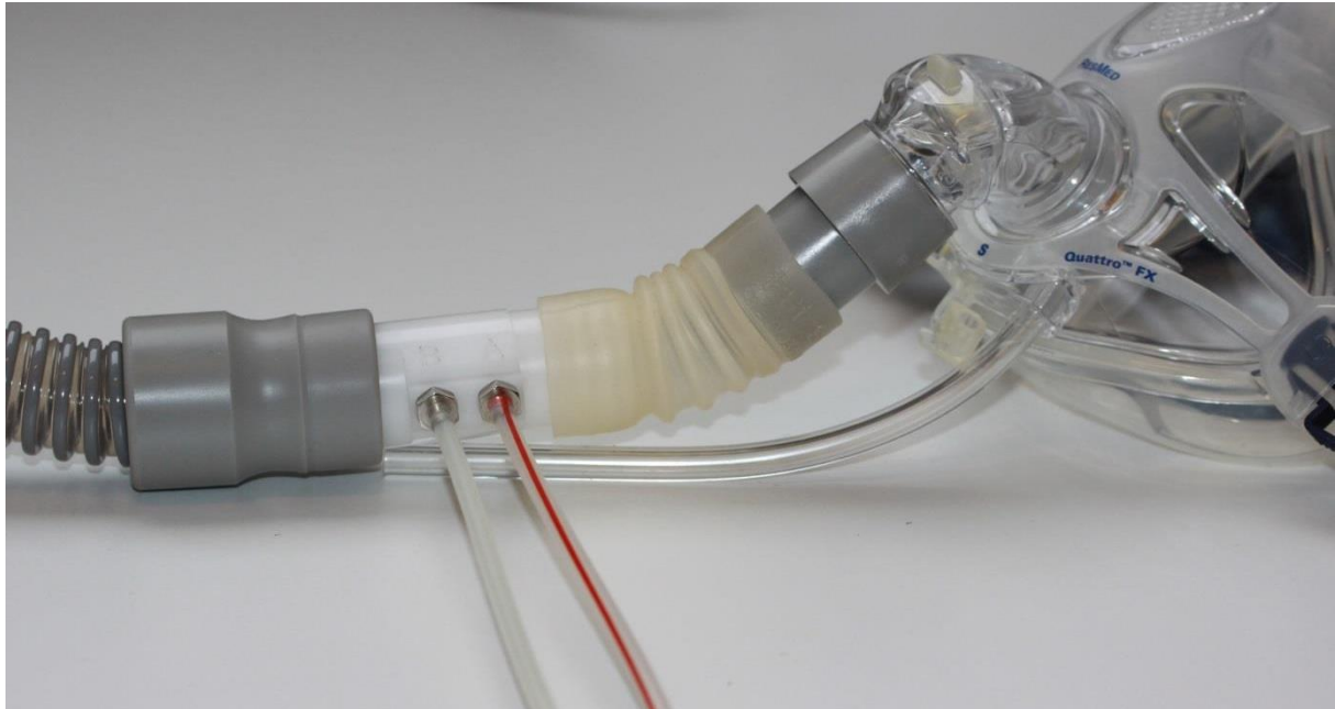
Figure 11. A tube connected to the oxygen port in the mask was used for mask pressure measurement. A pneumotachograph inserted in the ventilator circuit close to the mask for flow measurement in the circuit (Private photo).
