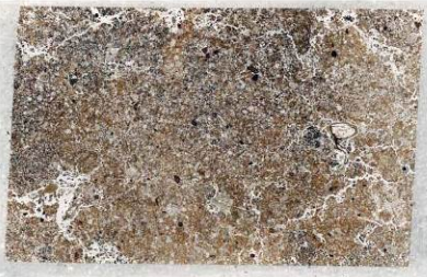
Fig. 26: Scan of M3987B (A1446); a highly mixed heterogeneous soil, with modern humic fine soil and rooting mixed into original compact soil. Frame width is ~75mm.
