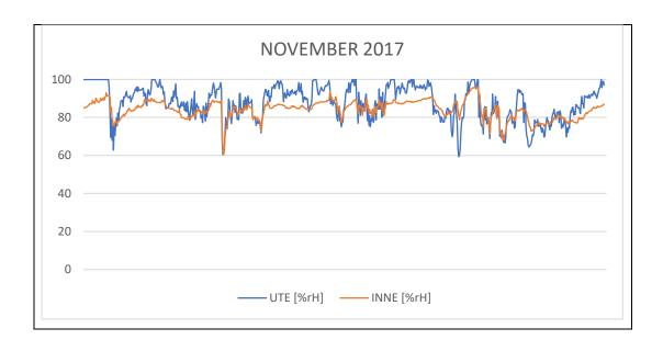
Figure 21. Humidity curves November 2017. Blue curve = outdoors, orange curve = indoors
