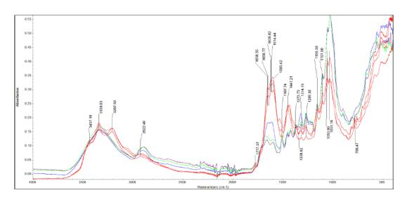
Figure 11. Effect of rinsing sample 6 (red spectra are before rinsing).
