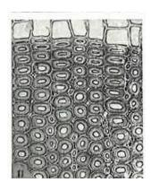
Figure 4. Cross section of a softwood, magnified 175x, showing rounded outlines of compression wood tracheids and associated intercellular spaces. (Phillips, 1948)
