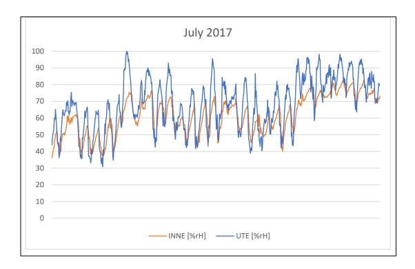
Figure 20. Humidity curves July 2017. Blue curve = outdoors, orange curve = indoors
