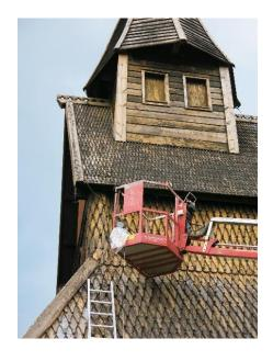
Figure 38. During X-ray examination of the SW corner. The X-ray generator was placed on an aerial lift, and the pictures were taken using a trigger button from the ground.
