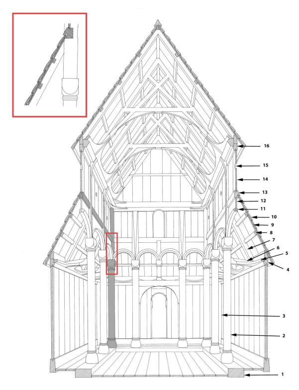
Figure 1 Two drawings of Urnes stave church, from Håkon Christie (2000). The SW nave corner post and bressummer in grey. Cross section of the aisle roof and bressummer inside the red frame.
