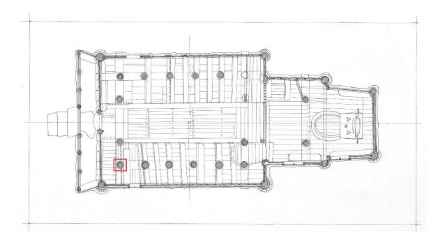
Figure 3. A plan of Urnes stave church, showing the posts. The SW nave corner post inside the red frame. Drawing by Einar Oscar Schou (1877-1966).
