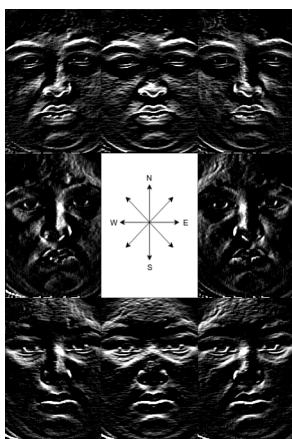
Fig. 10: Kirsch mask applied in all eight directions on a single grayscale image.
