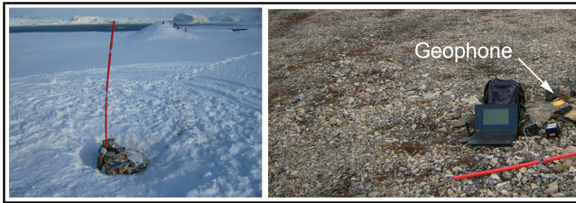
Figure A1. Photos of a station of the KBSA array after deployment in April and a station of the BRA array during data retrieval in August (geophone uncovered).
