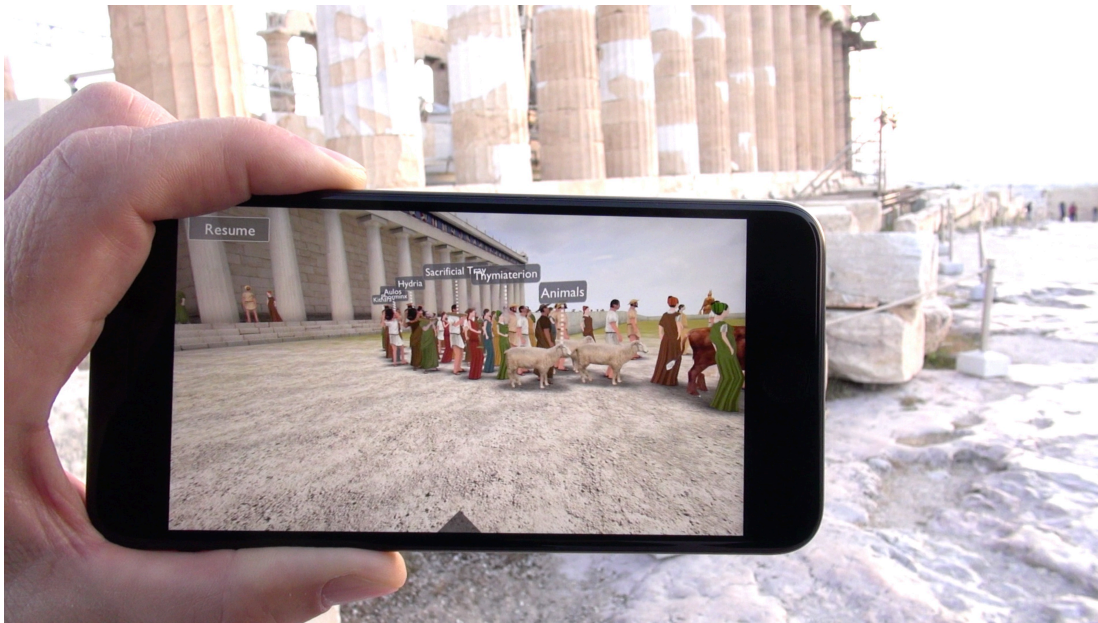
Fig. 5. A touch on the screen surface has halted the temporal sequence and animation and the information layer where spatially positioned hypertext links are visible. Links are attached to moving objects in the procession; animals, humans, instruments etc. The 'Resume' button in the upper left corner ends the pause mode and returns us to the animated sequence mode.
