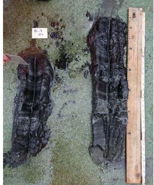
Figure 2.1b – One set of pseudo-replicates (BC-B) that have been sliced vertically and logged.
