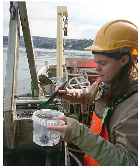
Figure 2.1c – Collecting sediment sample from the Van Veen grab.
