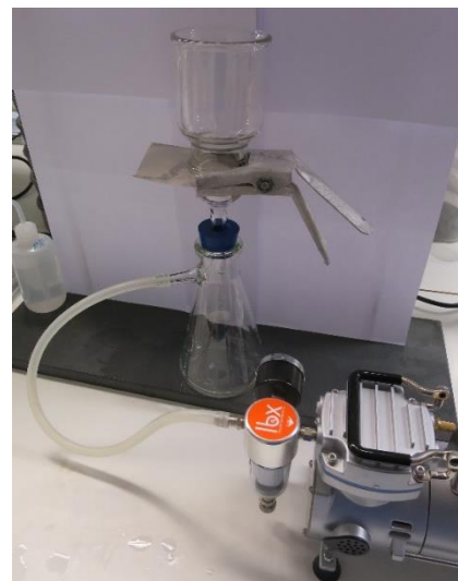
Figure 2.7c – The filtration setup. Sample material was collected onto a steel mesh filter by using a vacuum filtration system.
