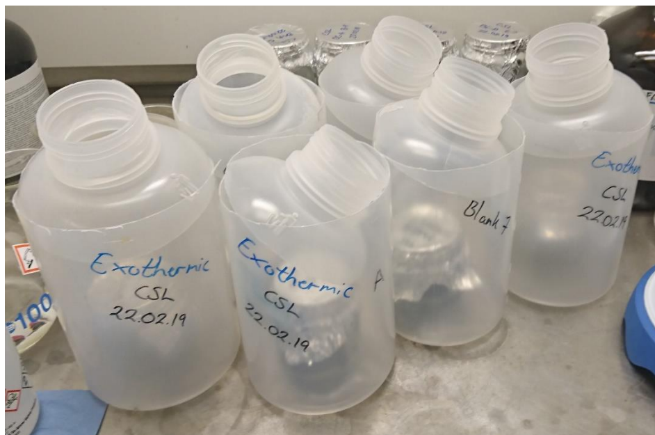
Figure 2.8b – Step 2 of chemical digestion. The samples in the glass jars have been placed in tall plastic (PP) containers.
