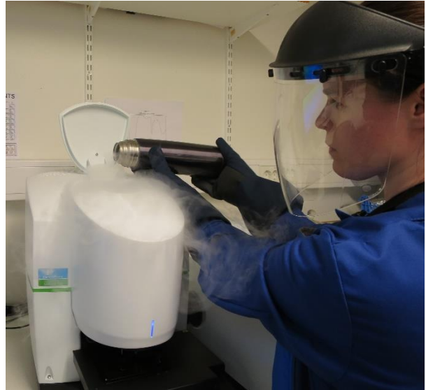
Figure 2.11b – The FT-IR Microscope Spotlight 200i had to be filled with liquid nitrogen before use.
