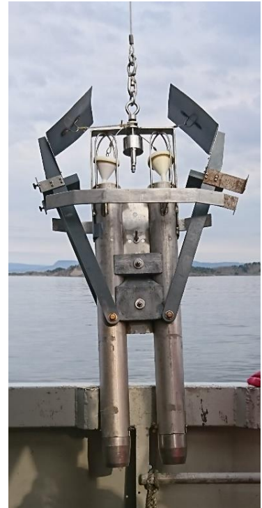
Figure 2.1a – A Gemini corer ready to collect sediment.
