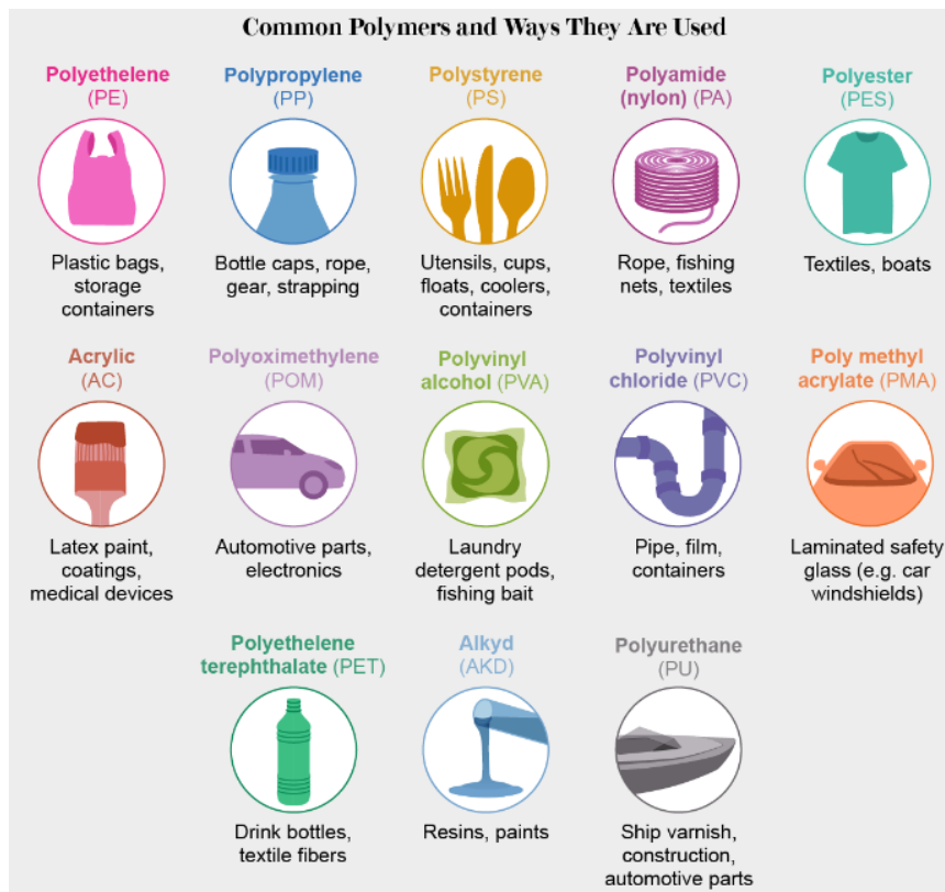
Figure 1.2 – Common plastic types and examples of products that are made of the different types (Thompson, 2018).
