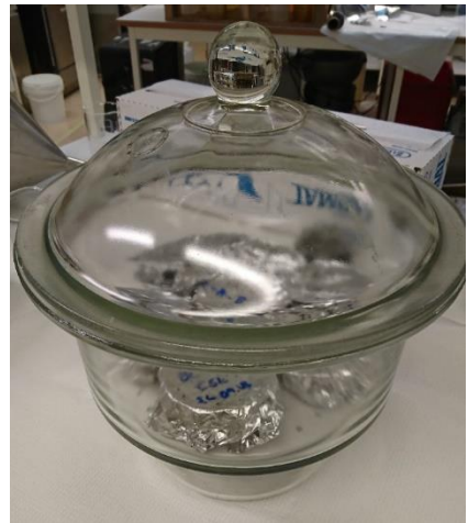
Figure 2.8c – Desiccator with a few samples that have been through chemical digestion.
