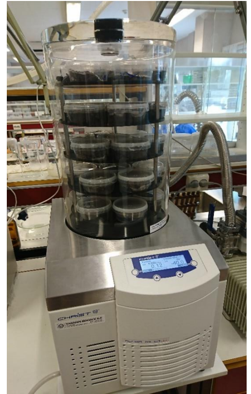
Figure 2.2 – Freeze dryer with 35 samples inside, ready to be dried.
