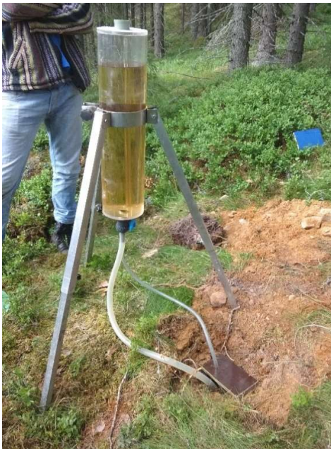
Figure 8. Mariotte cylinder infiltration test conducted in Elverum.
