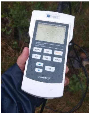
Figure 20 VWR PC 5000 L electrical conductivity meter
