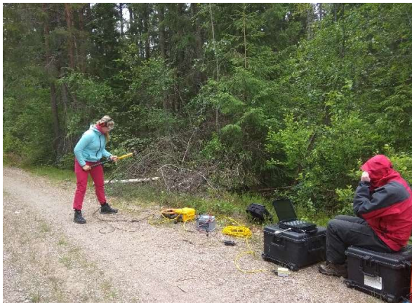
Figure 15. Seismic refraction survey in one of the locations in Grindalsmoen.
