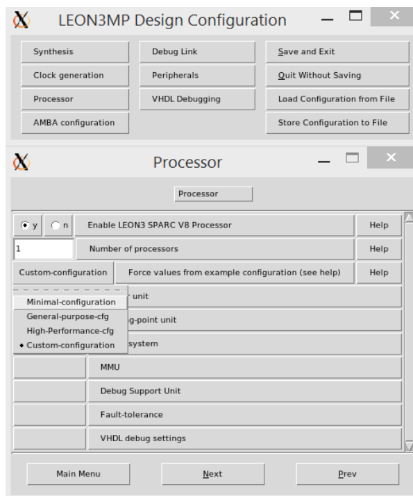
Figure 11: LEON3 custom configuration setup with Xconfig
