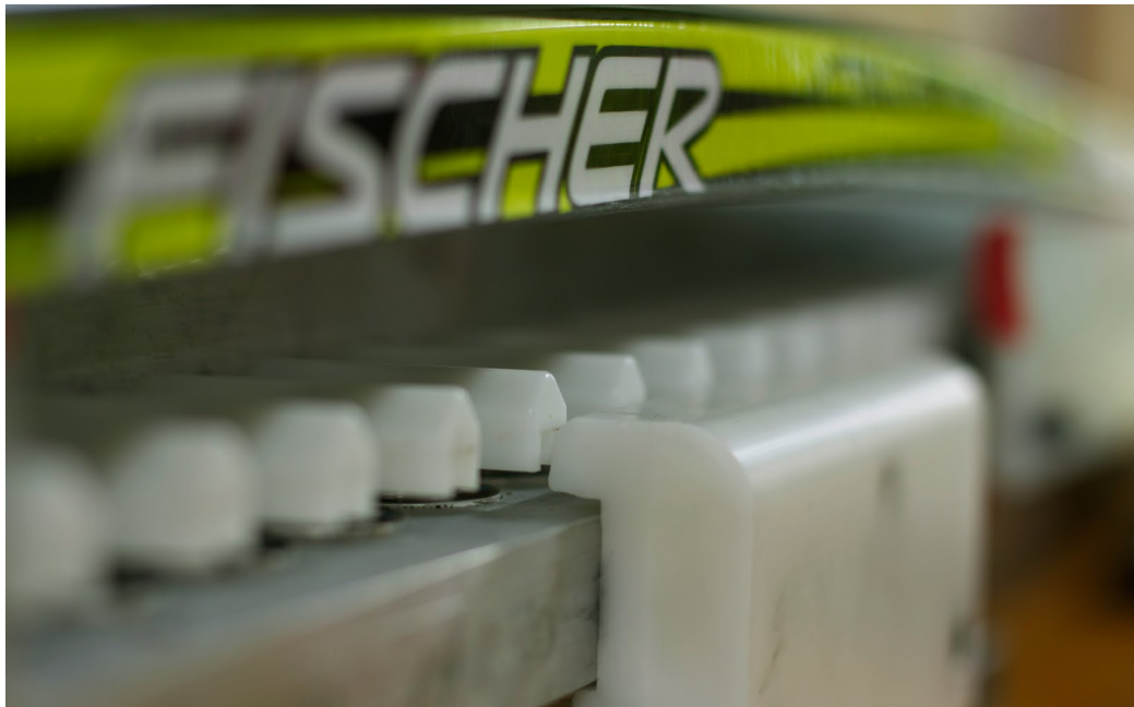
Figure 2.8: Figure show a ski placed ontop of the Gear West Signature Flex tester, image taken from Gear West (2011).
