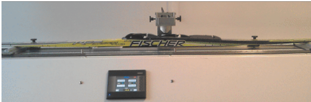
Figure 2.3: Ski test bench developed by Felix Breitschädel. Figure from Breitschädel (2014).
