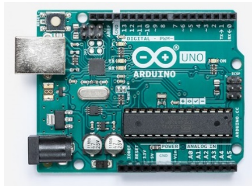
Figure 6.2: Arduino Uno Rev3 MCU. Figure taken from Arduino AG (2019).
