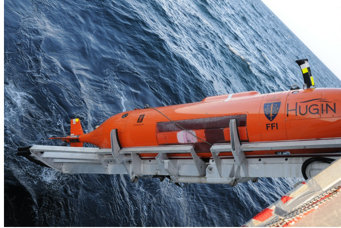
Figure 2.1: Image of a HUGIN AUV equipped with HISAS 1032 interferometric SAS from the FFI research vessel H. U. Sverdrup II during the Marex17 scientific trials outside Bergen, Norway, in March 2017. The HISAS is the brown rectangular objects forming a "H"-looking shape mounted on HUGIN. Photo courtesy of FFI and used with permission.
