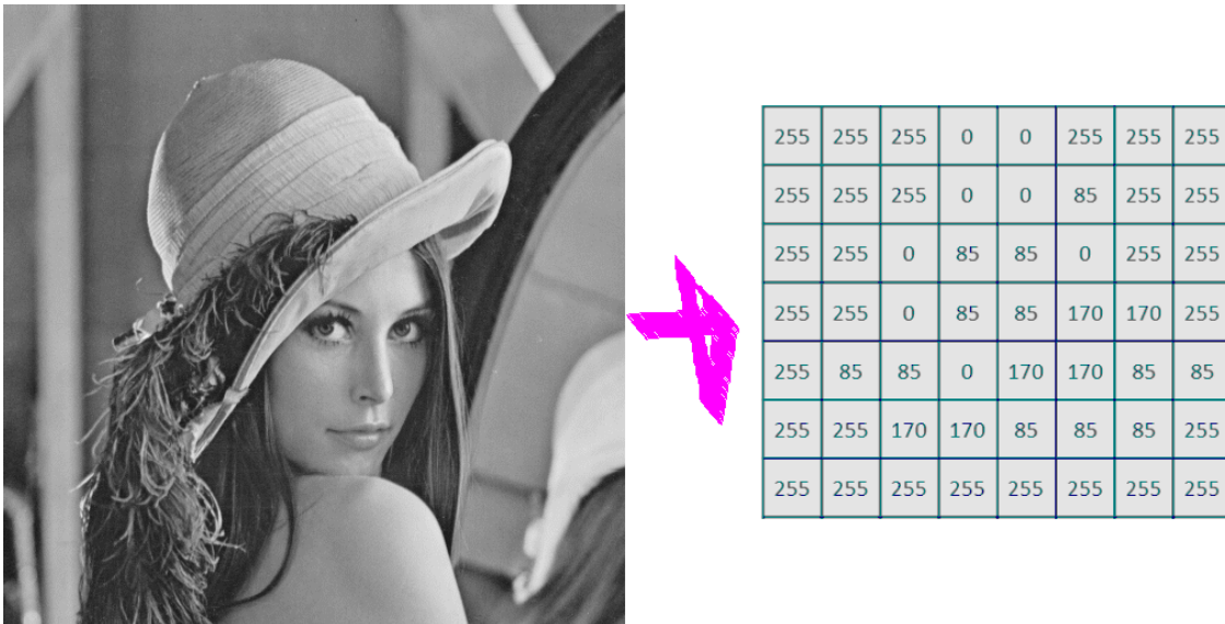
Figure 5.1: A grey scale image can be represented as a matrix with pixel values between 0 and 255, where 0 represents black and 255 represents white.
