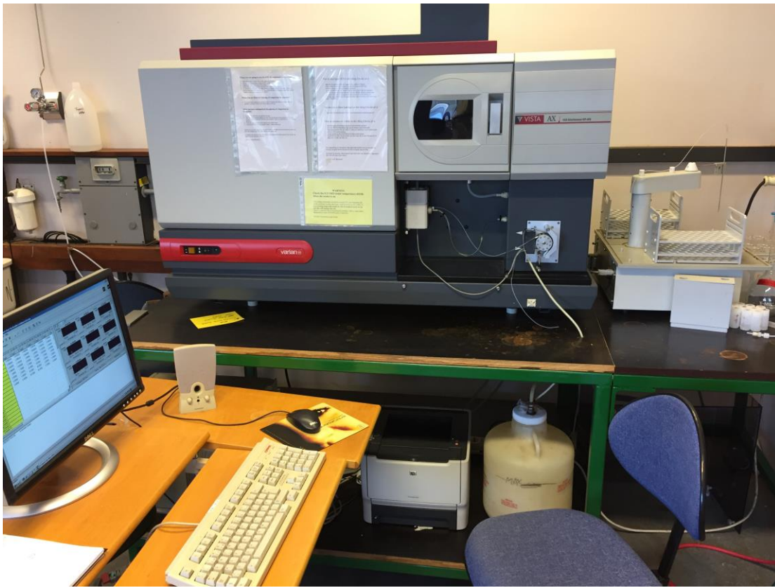
Figure A.10: Major cations were analysed using this Varian Vista AX CCD simultaneous ICP-AES instrument.
