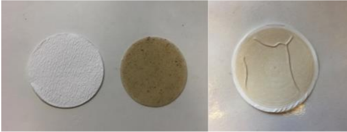
Figure 3.2: Filters used to filter spring outlet samples. The filter to the right is a glass fibre filter before filtration. The filter in the middle is taken after filtering raw outlet water through 0.7 µm. The filter to the right is a cellulose acetate filter after filtration of 0.7 µm water through 0.2 µm.
