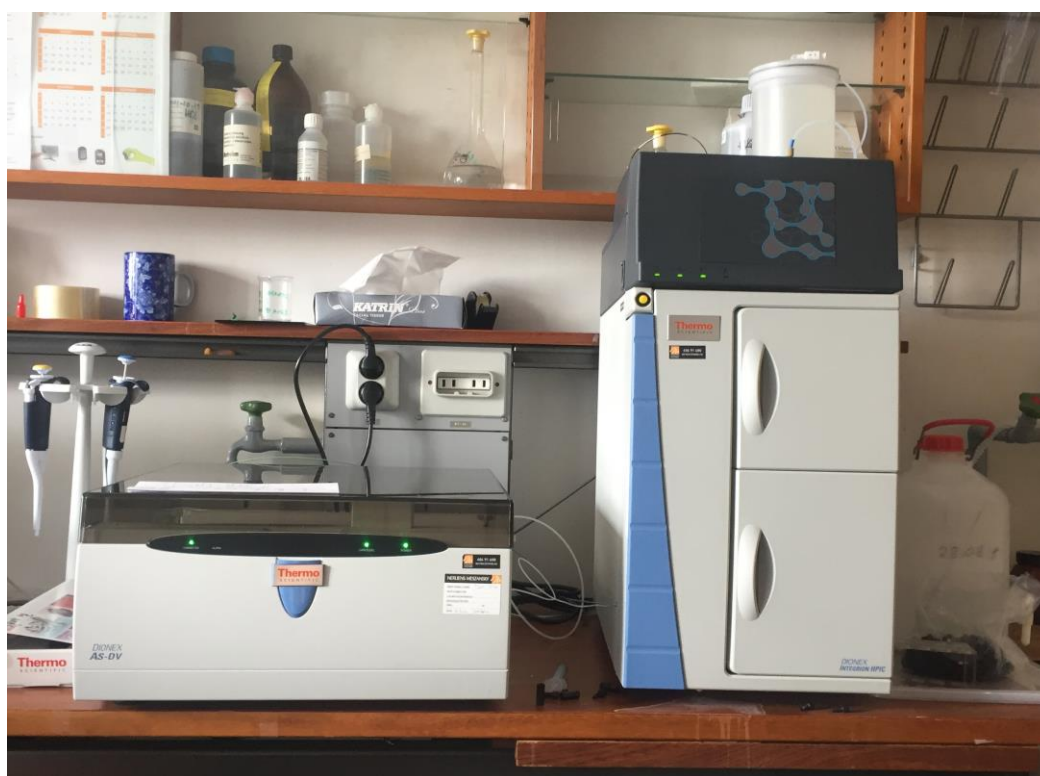
Figure A.8: Major anions were analysed using this Thermo Scientific Dionex Integriion HPIC instrument with a Dionex AS-DV autosampler. A computer connected to the instrument is used to run the software Chromeleon
