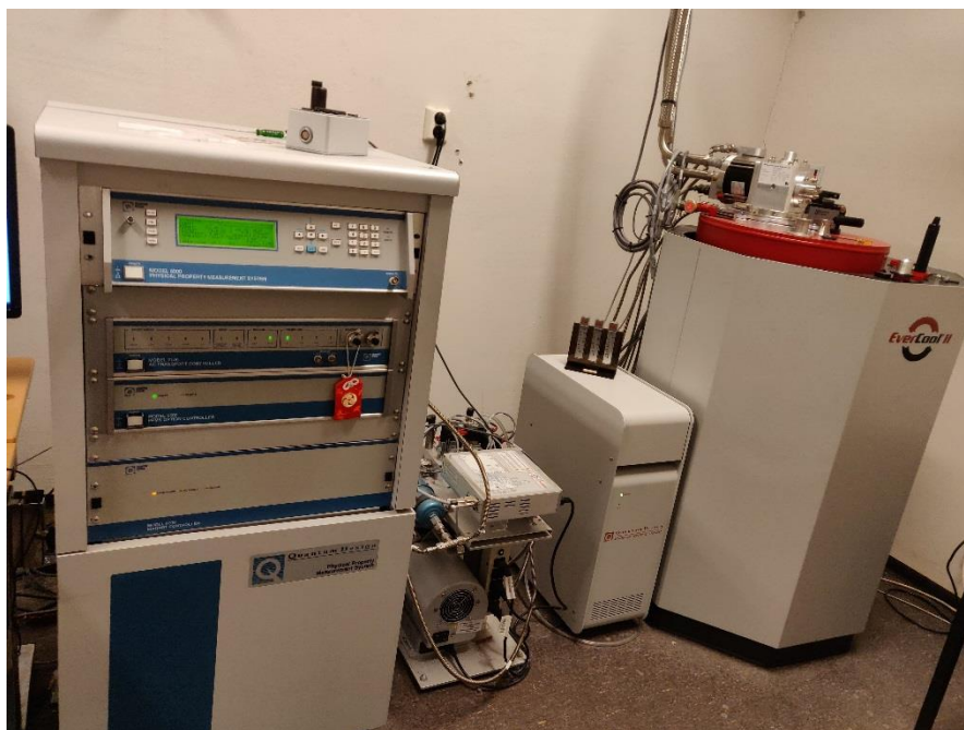
Figure 3.3-5: A photo of the PPMS-instrument used in this thesis (Quantum Design® Property Measurement System).
