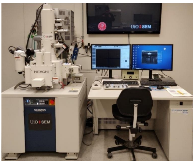
Figure 3.3-1: A photo of the SEM-instrument used in this thesis (Hitachi SU8230 Ultra High Resolution Cold FEG-SEM).
