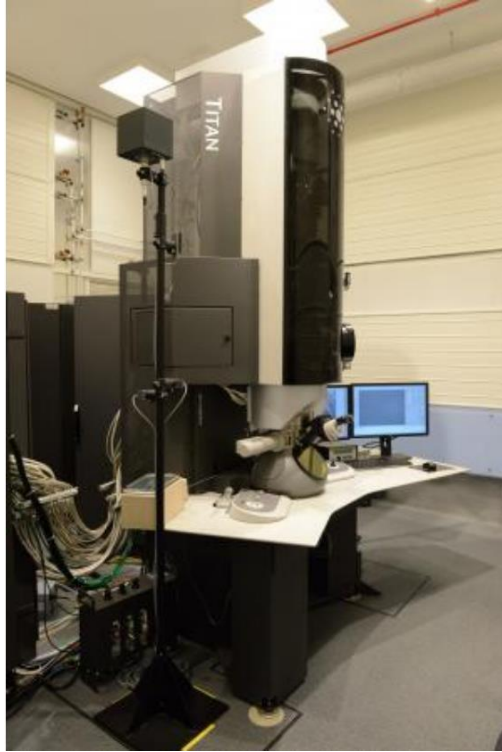
Figure 3.3-2: A photo of the TEM-instrument used in this thesis (FEI Titan G2 60-300 kV). The photo is taken from reference [75].
