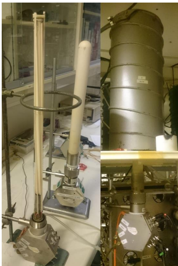
Figure 4.3: Left: The cell; without the alumina cover (in front) and with the alumina cover (back). Right: The cell sitting inside the tubular furnace, connected to the Solartron 1260 (black wires), temperature controller (orange wire) and to the gas mixer (copper tubes).
