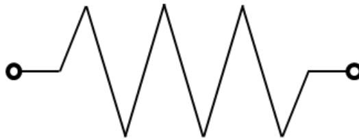
Figure 2.2: The symbol of a resistor in a circuit.
