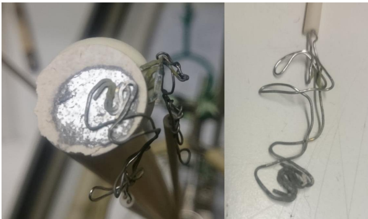
Figure 6.2: The corroded Pt-wire from measurement series 2. In the picture to the right the darker area at the folded part of the wire is the corrosion. This area is \text{Li}_2\text{PtO}_3 , which is a poor conductor.
