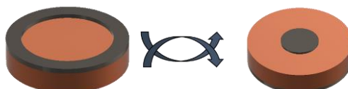
Figure 4.1 Schematics of the button electrolyte pellet (BZCY) with a platinum reference electrode (left) and counter electrode (right) painted on the electrolyte surface.
