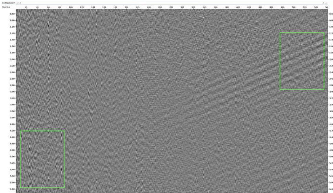
Figure 2.5: Tugging noise in seismic data. There is tugging noise present both from vessel and tail buoy marked in green squares
