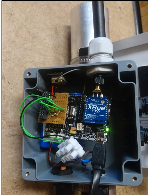
Figure 11: Picture showing the inside of the box holding the Waspote and the battery.
